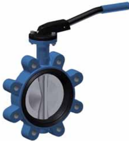
Butterfly valve with hand lever PN10/16 (DN40 – DN200)
